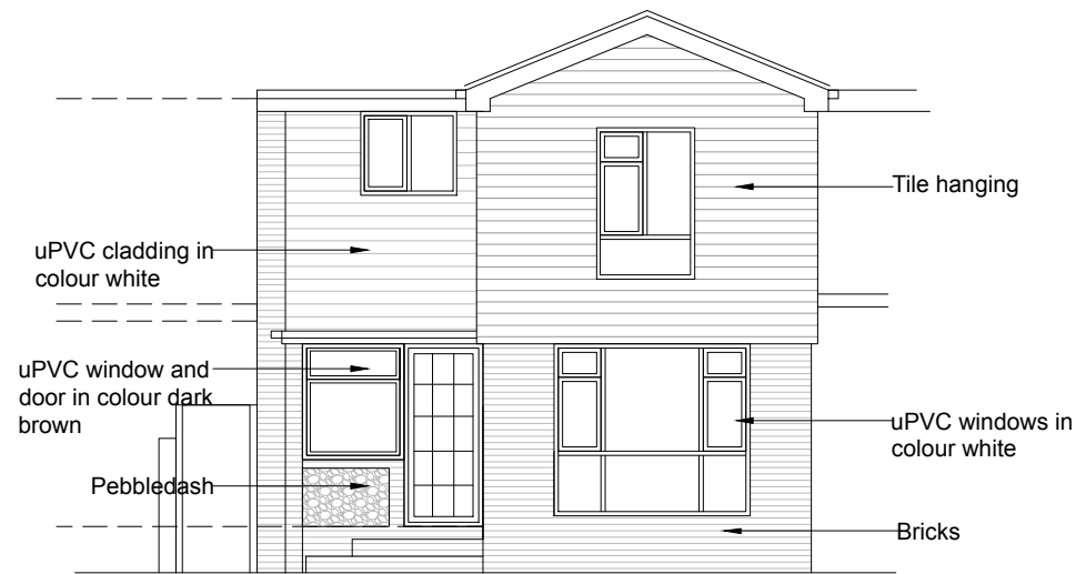
Front (North West) Elevation as existing
