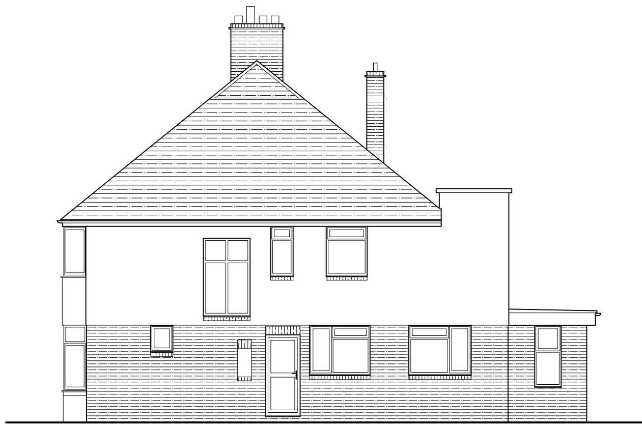
Proposed Side (north) Elevation Scale 1:100
