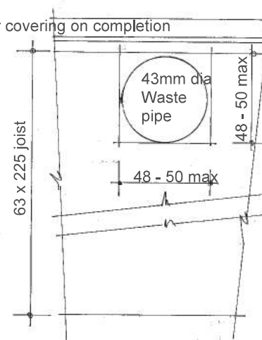
Waste pipe thro' floor joists 1:20
