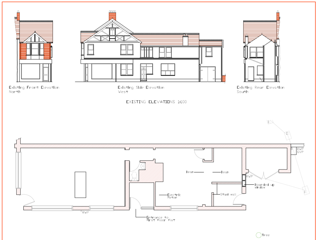
Figure 2: Existing ground floor plan and elevations (Source: BPM Architectural Services)
