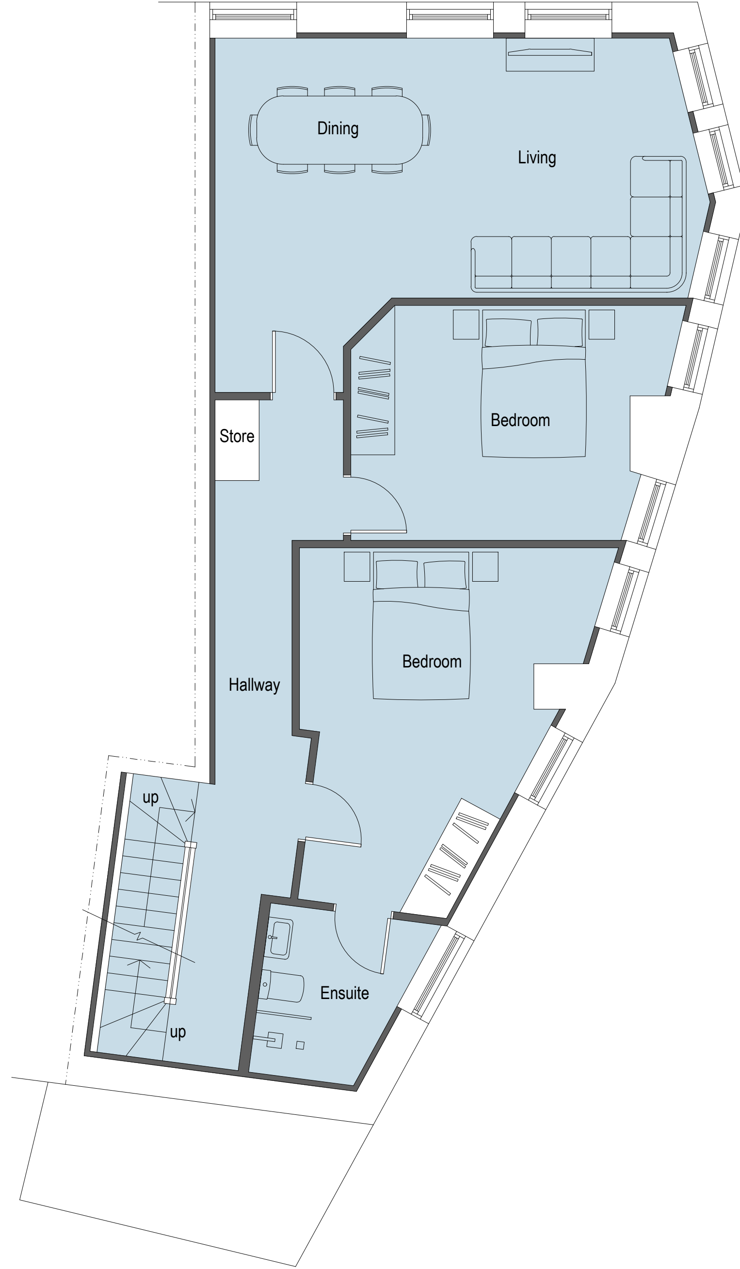
Proposed First Floor Plan 1:50
