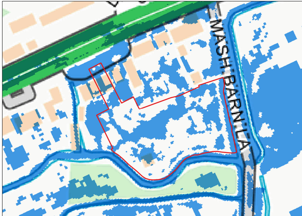
Figure 5.1 – Extent of flooding during the design pluvial event for the baseline conditions, as modelled by HCL (© Herrington Consulting Ltd and contains Ordnance Survey data © Crown copyright and database right 2025).
