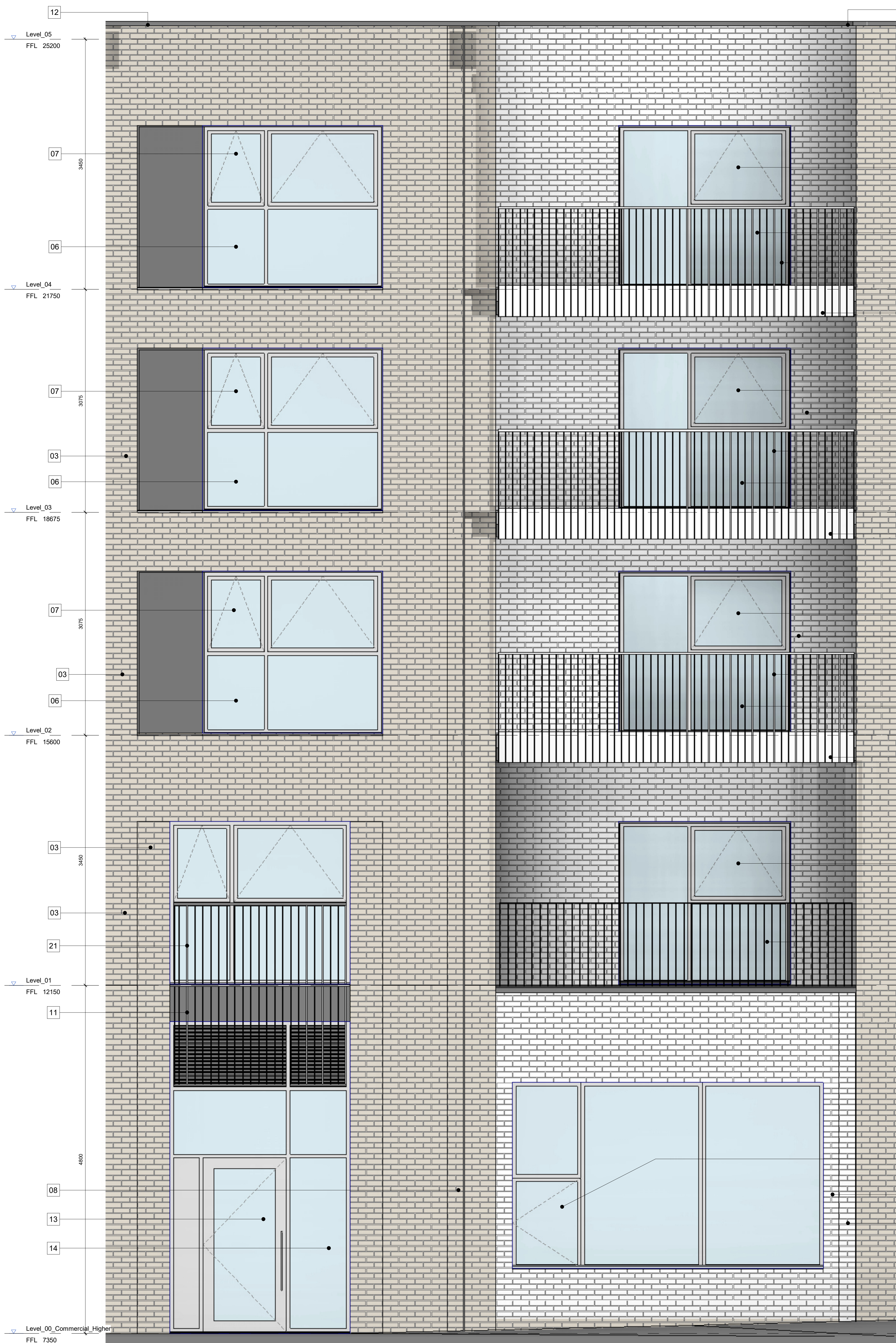
1 EAST ELEVATION HIGH ST BLOCK A 1 : 25
