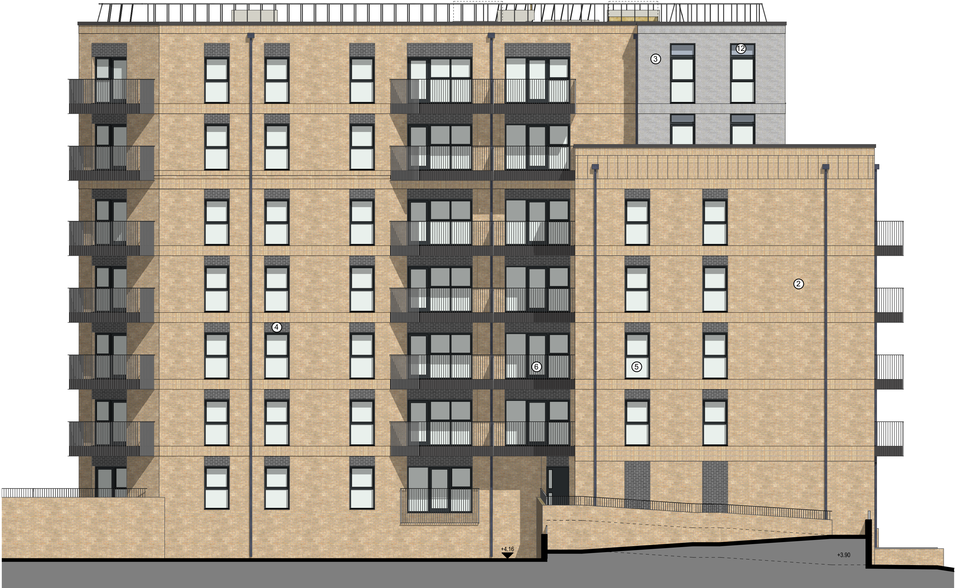
2 Building 3 Planning East Elevation 1:100
