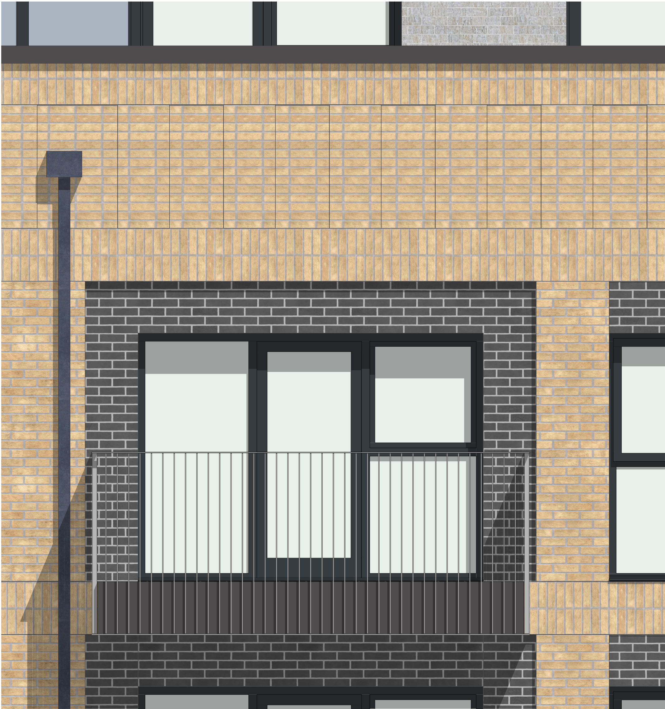
2 Inset balcony elevation (Building 03) 1:20
