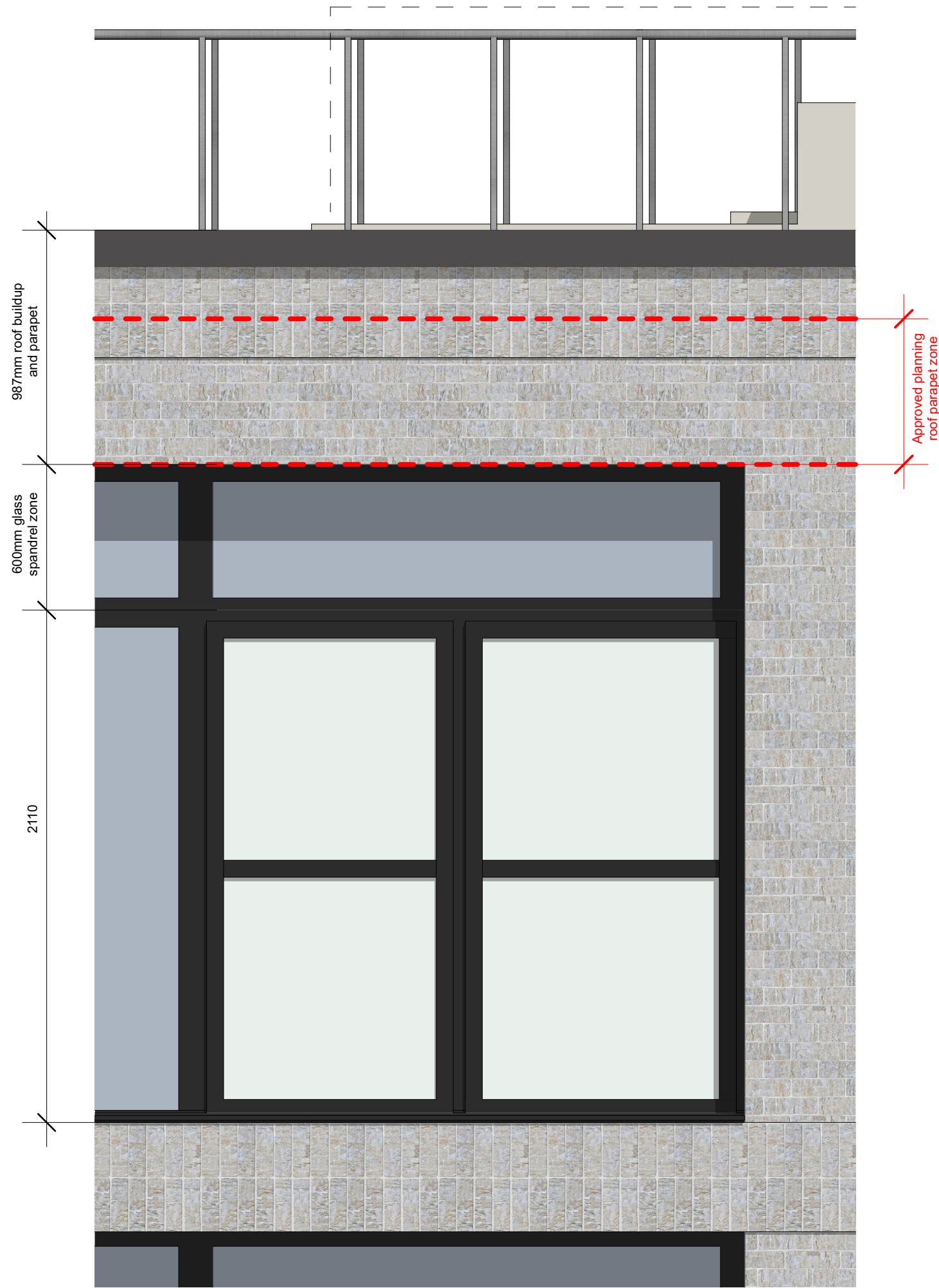
2 Building 02-03 Top floor Elevation 1:20
