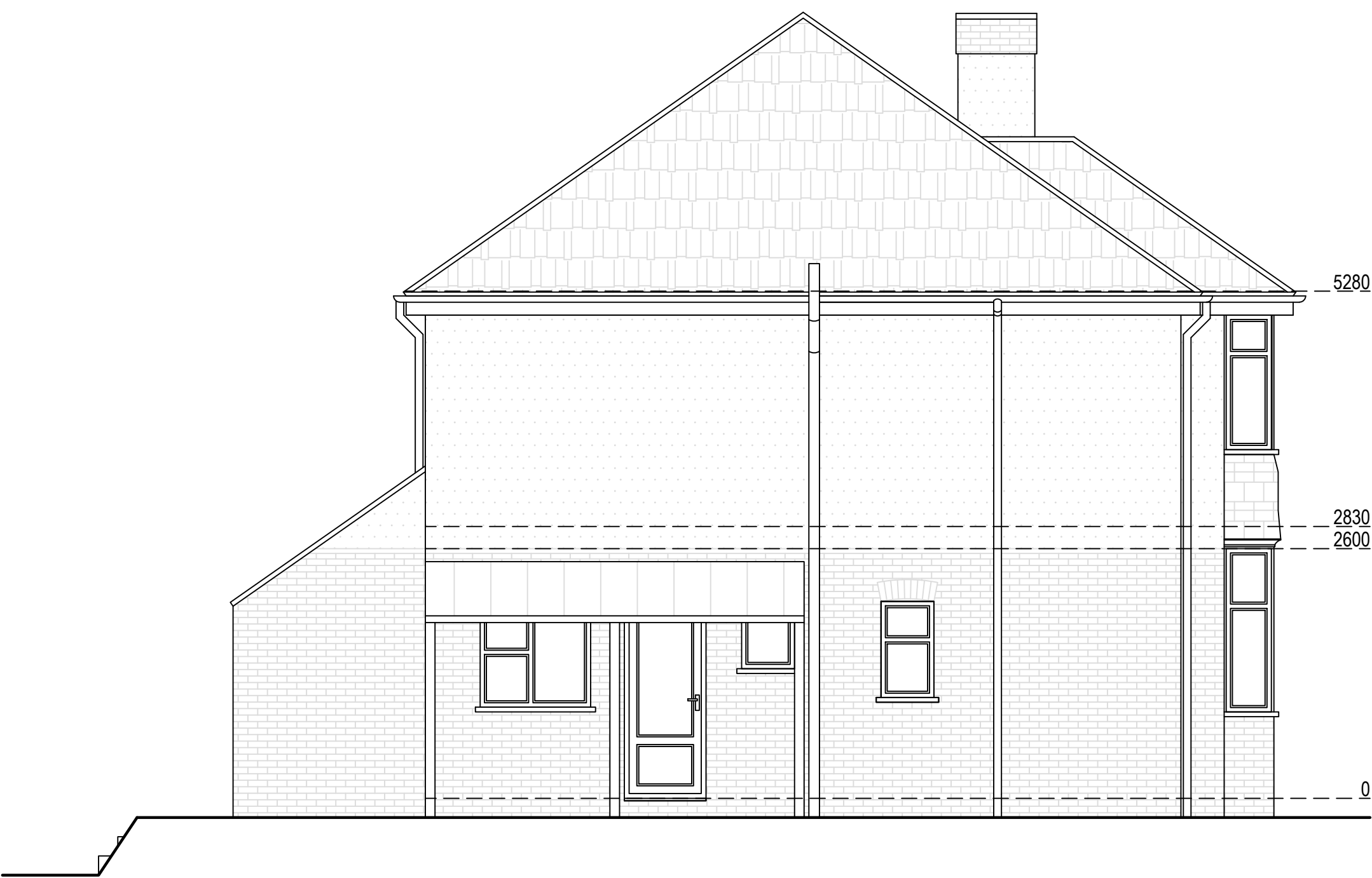
Existing East Elevation
