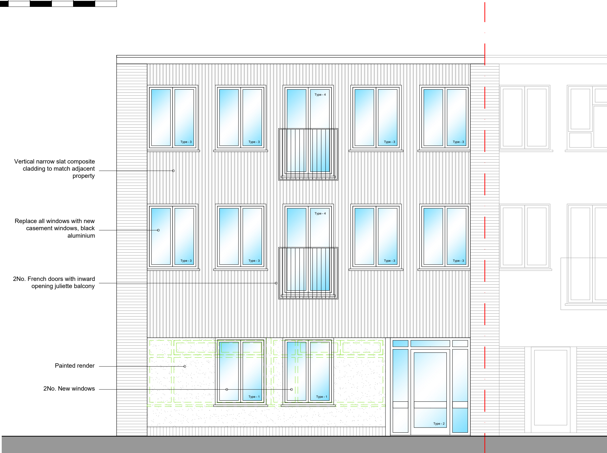
Proposed Front Elevation (South East) 1:50 @ A1
