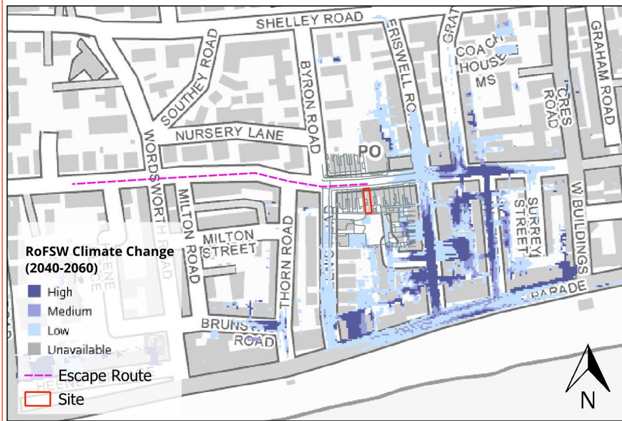
Figure 21: Potential route of safe egress through surface water with reaching or exceeding 0.75 flood hazard rating (Source: EA, OS)
