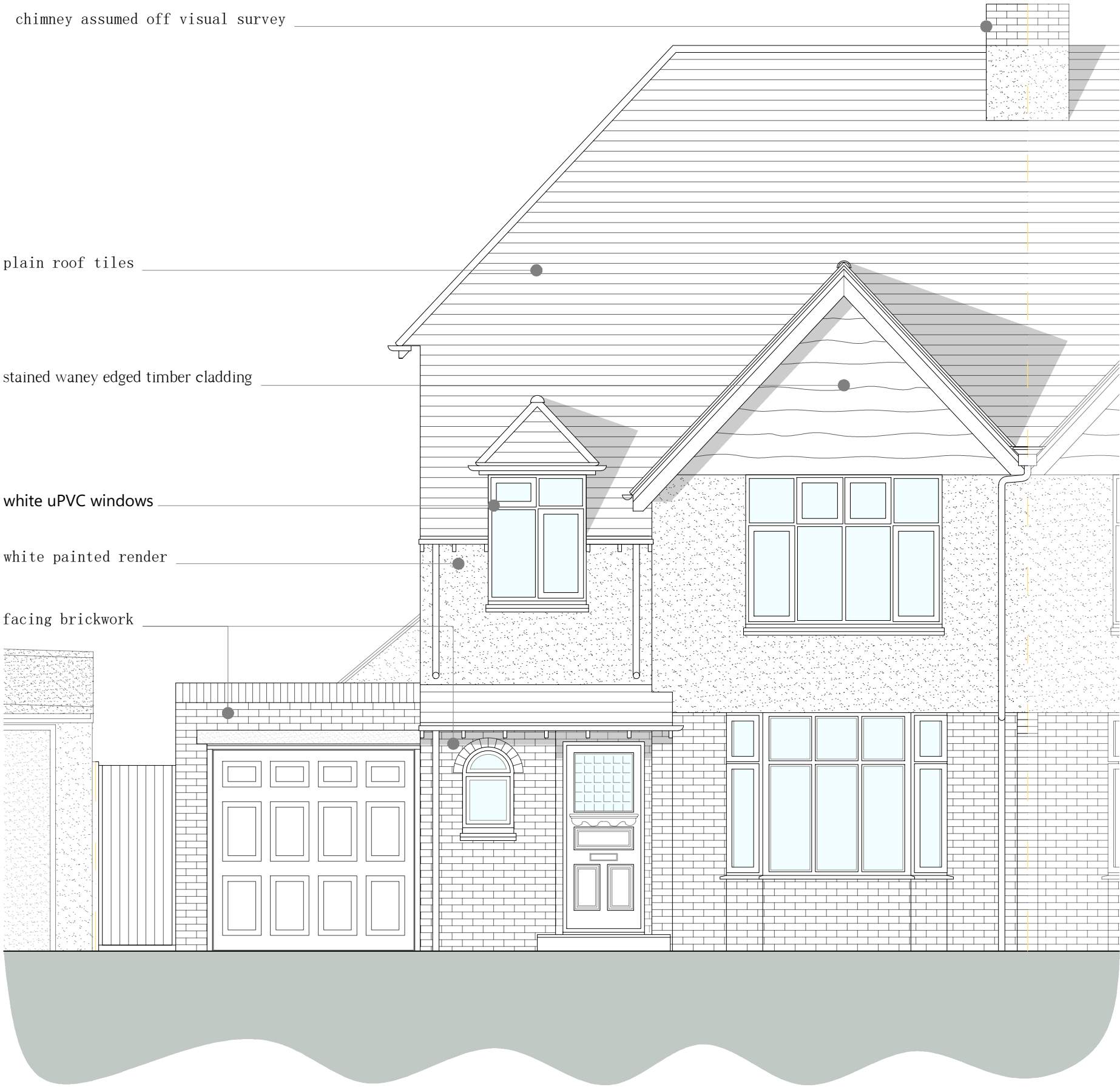
existing west elevation 1:50
