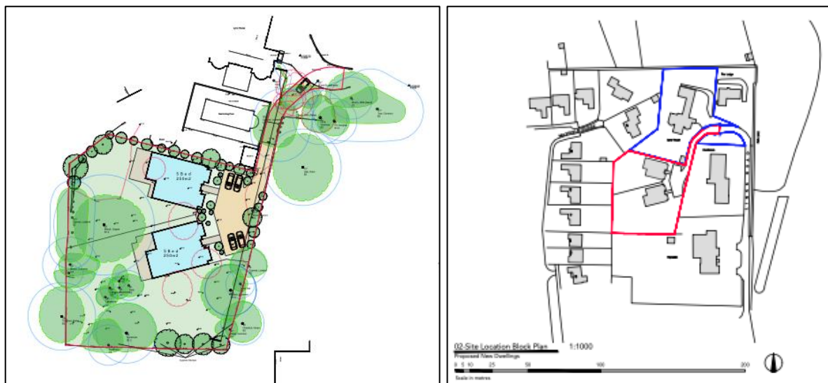
Figure 2. Proposed development layout plan for two new residential dwellings south of Lyne House, Worthing. Image courtesy of Architectural Design LLP, drawing number 2194(11)001. Right, red line indicates redline
