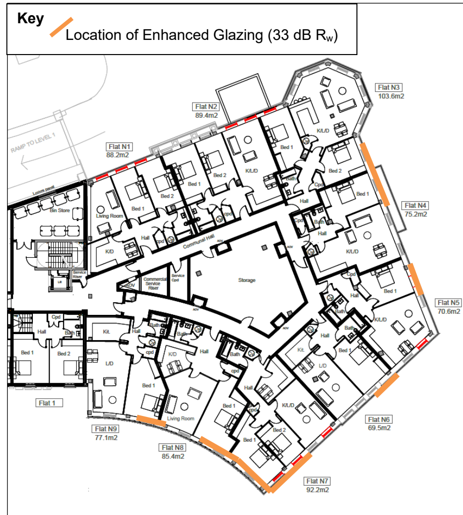
Figure A8 : Locations of Enhanced Glazing System
