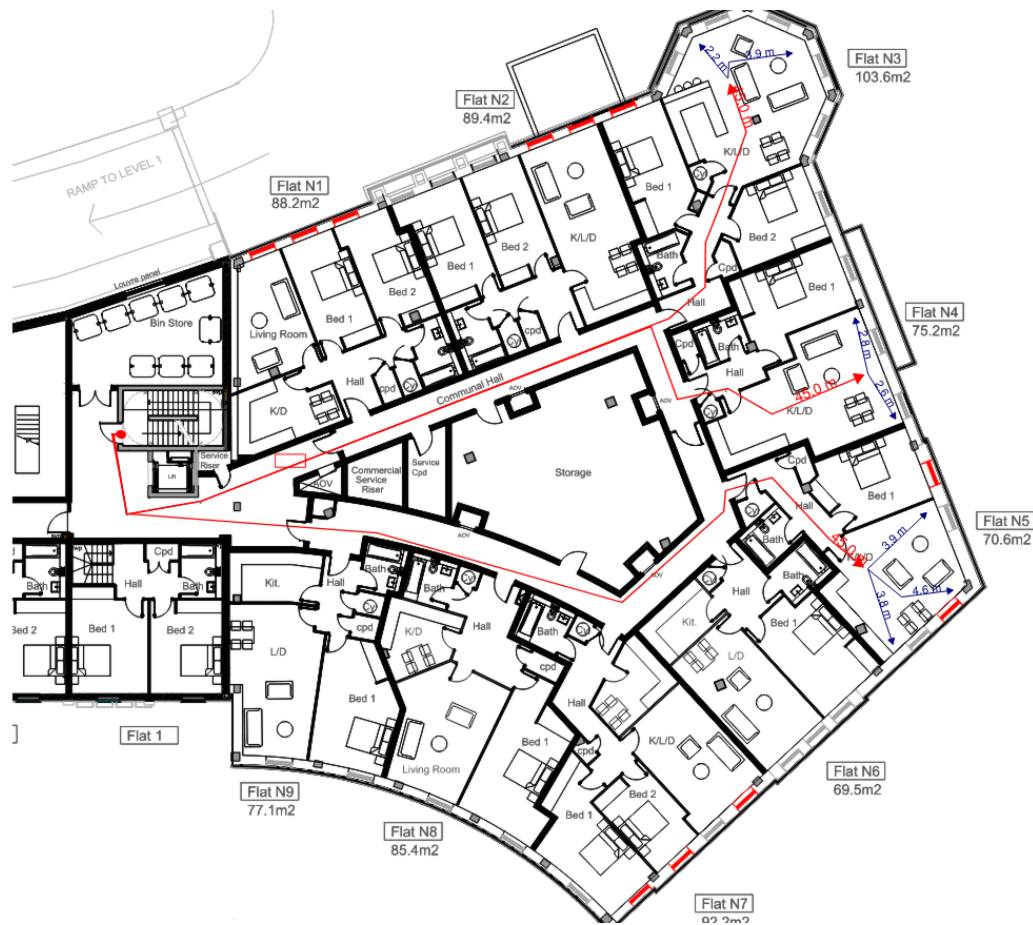
Figure 9: Hose laying distance.
