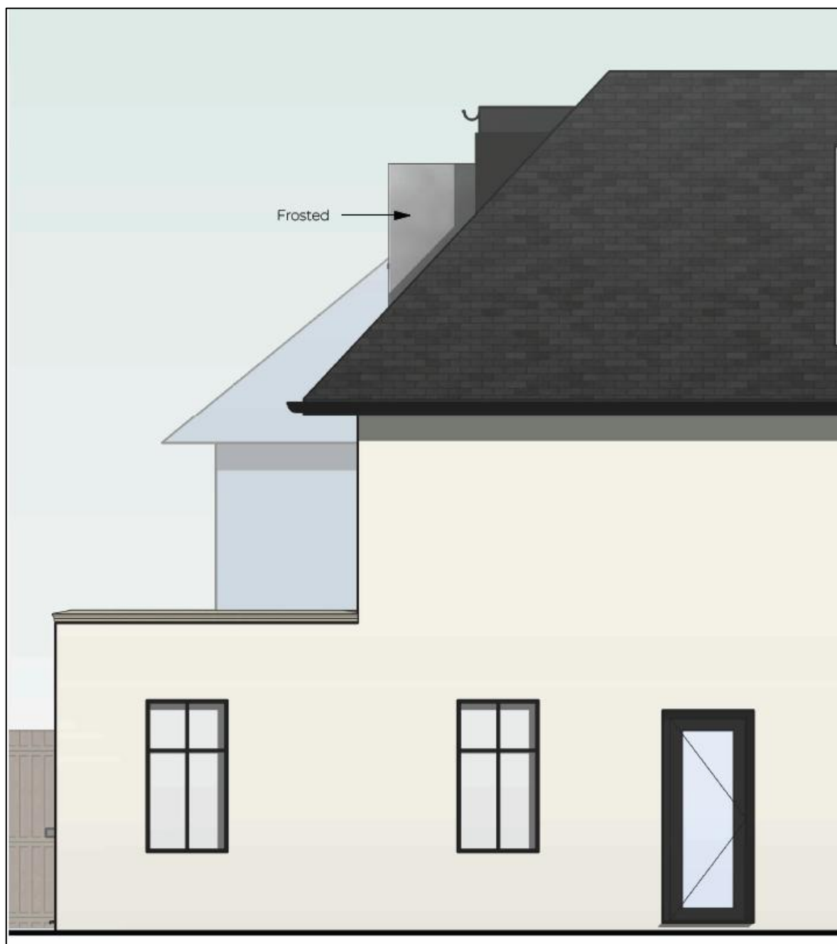
Figure 21 - Proposed Roof Terrace Privacy Screening
