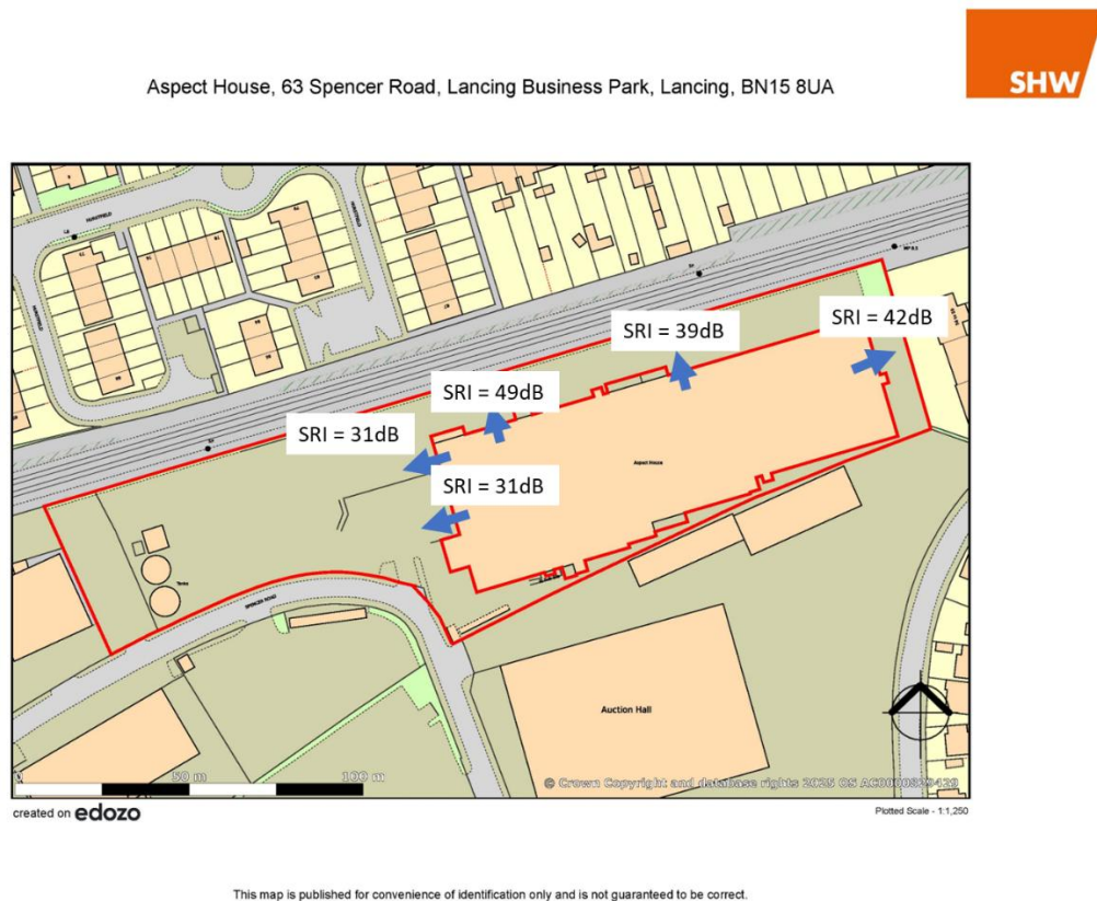
Figure 6: Sound Insulation of Aspect House Façade
