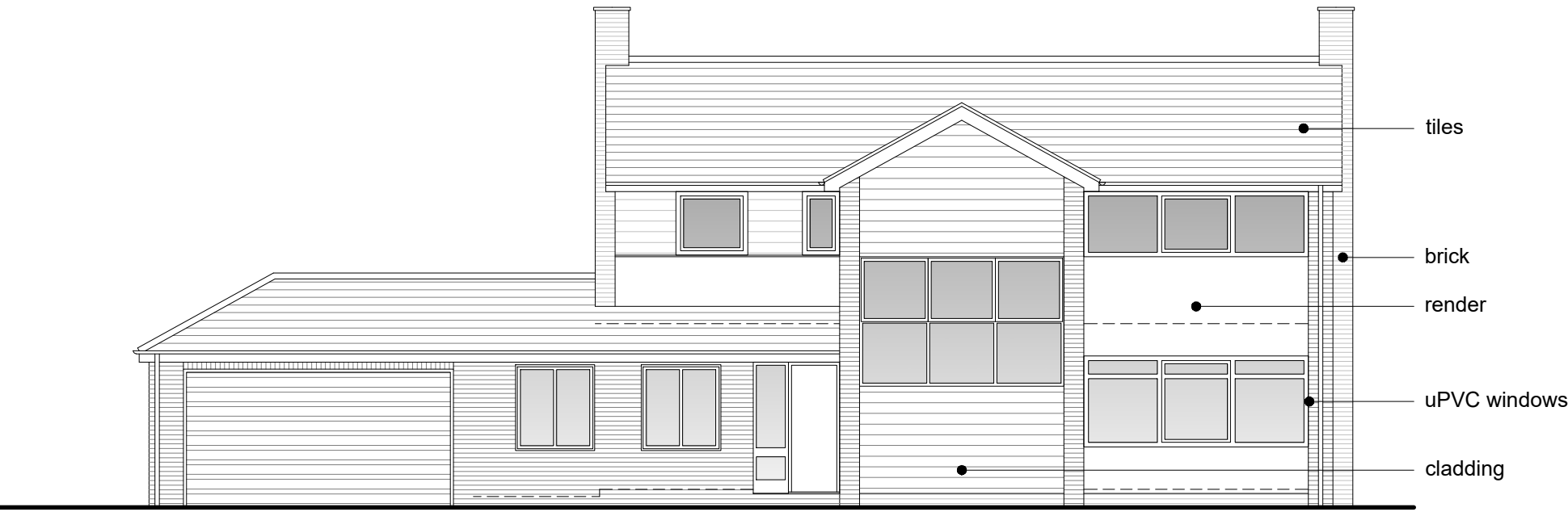
Existing Front Elevation (North-East) 1:100
