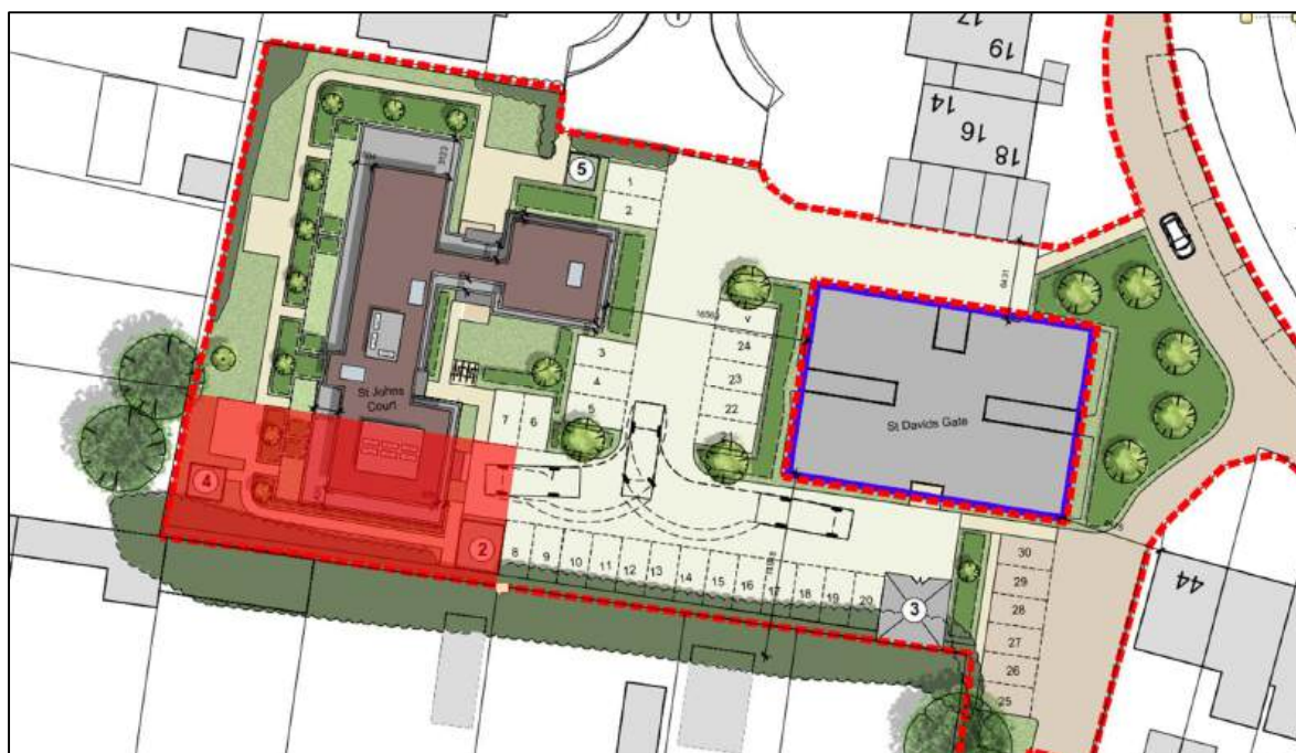
Figure 2.2 – Area of existing hardstanding to be removed
