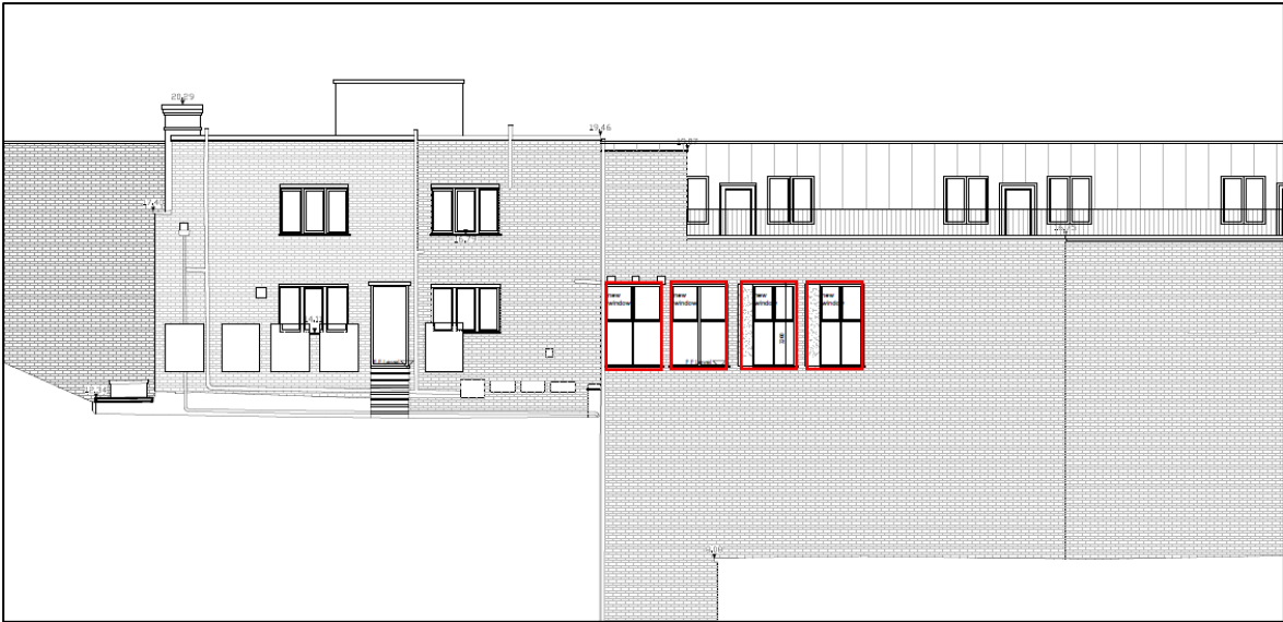
Proposed Eastern Elevation showing new windows at second floor level outlined in red.
