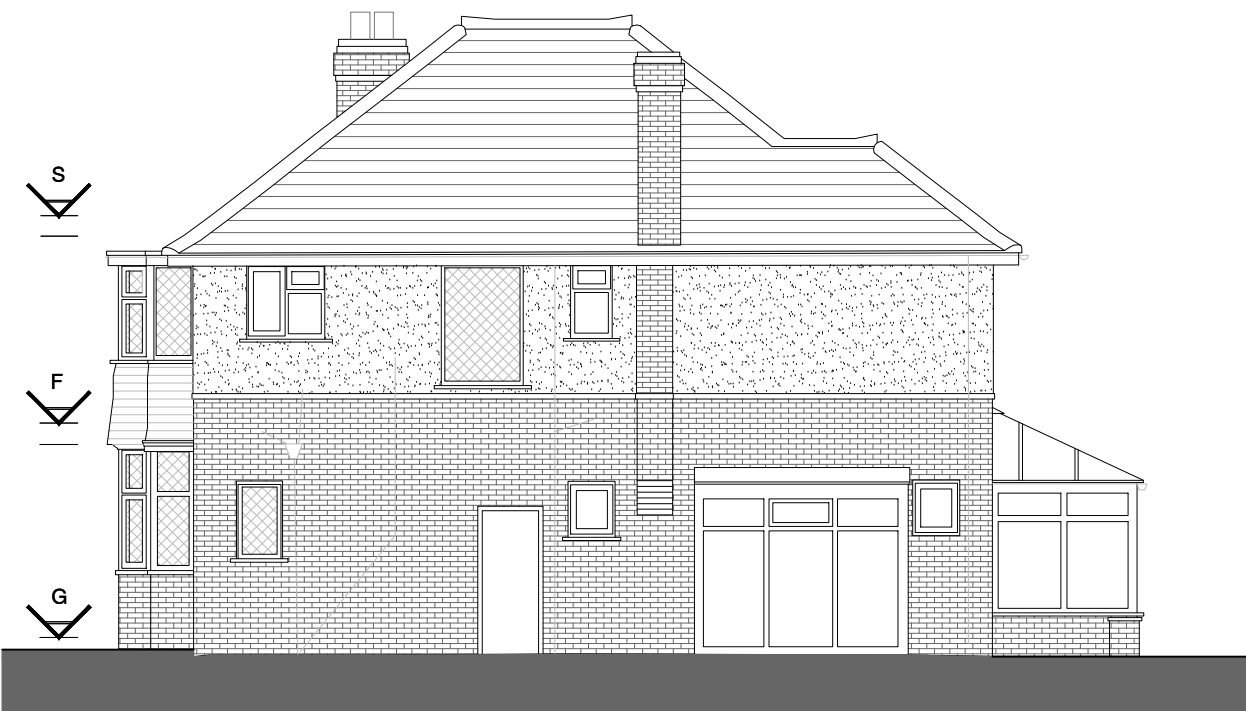
07 | EXISTING SIDE ELEVATION (WEST FACING) 1:100
