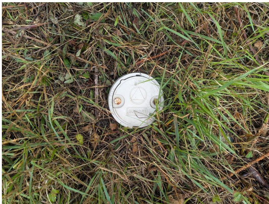
Photo 20. Monitoring borehole observed in the south of the Site.
