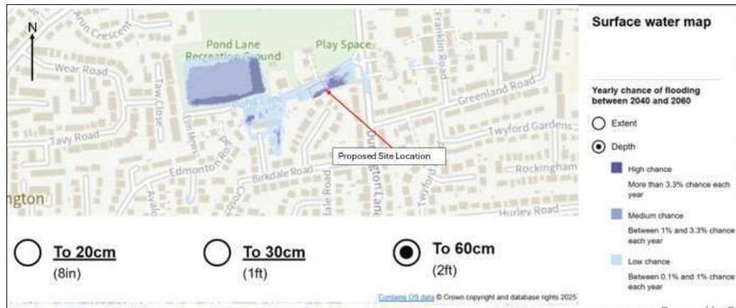
Figure 5-4 Long-Term Flood Risk Map: Surface water showing that parts of the south of the site has a “High Chance” of flood depths of up to 60cm
