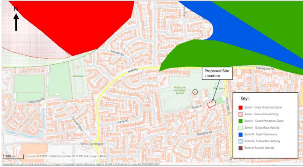
Figure 4-4 Proposed site relative to nearby Source Protection Zone (SPZ) (source: DEFRA Magic Map)
