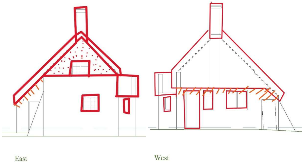
Figure 5. Existing East & West Elevations – repair (orange) or reinstate to replicate pre-fire (red)
