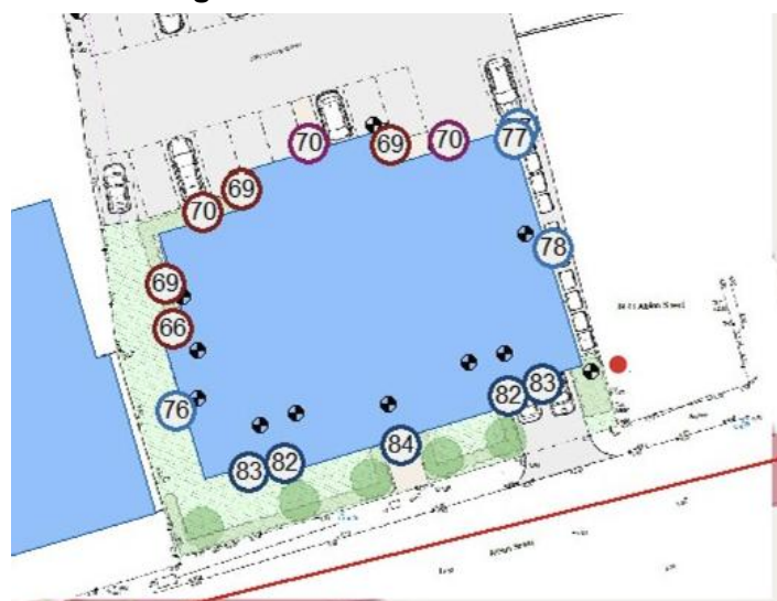
Nighttime LMax Third Floor
