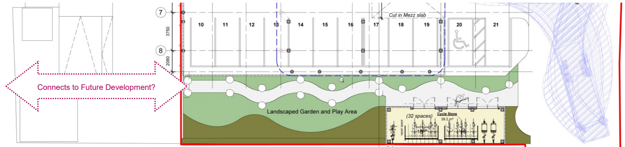
Bike Store is relocated along the south boundary, with the area west redeveloped as a private amenity space for residents - either exclusively for this development, or in conjunction with the future development adjacent
