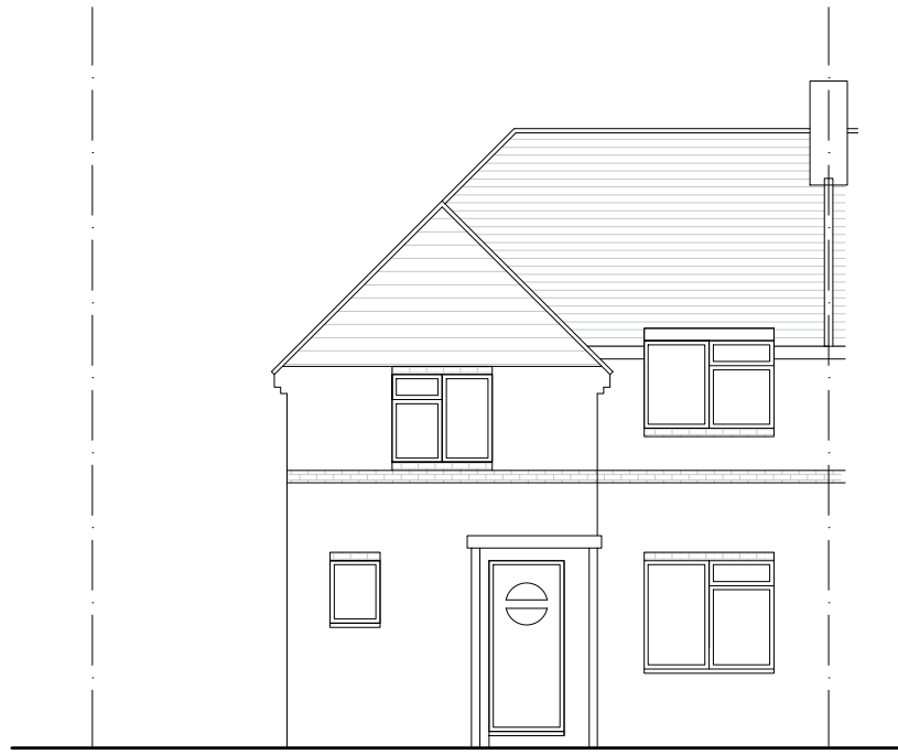
EXISTING FRONT ELEVATION (N) 1:100
