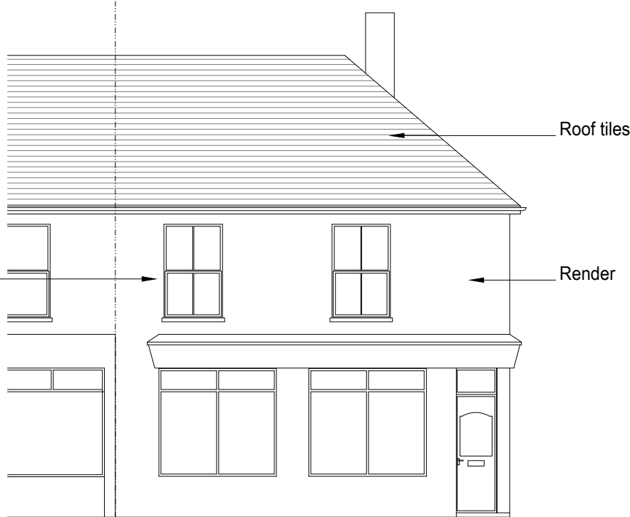
Existing Front Elevation (North) 1:100
