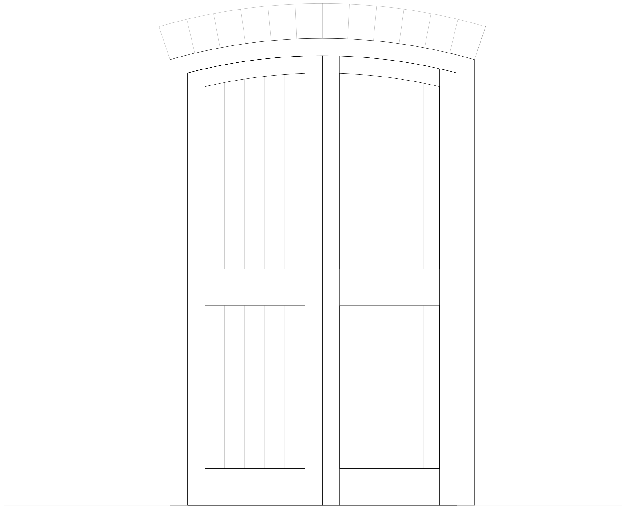
South Entrance Door- Internal elevation 1:10 | PROPOSED
