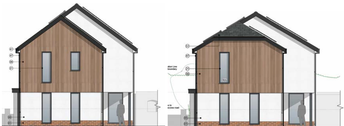
Figure 02. West Elevation: Pre-app scheme (left), revised scheme (right)
