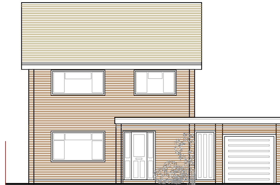
PROPOSED NORTH ELEVATION 1:100
