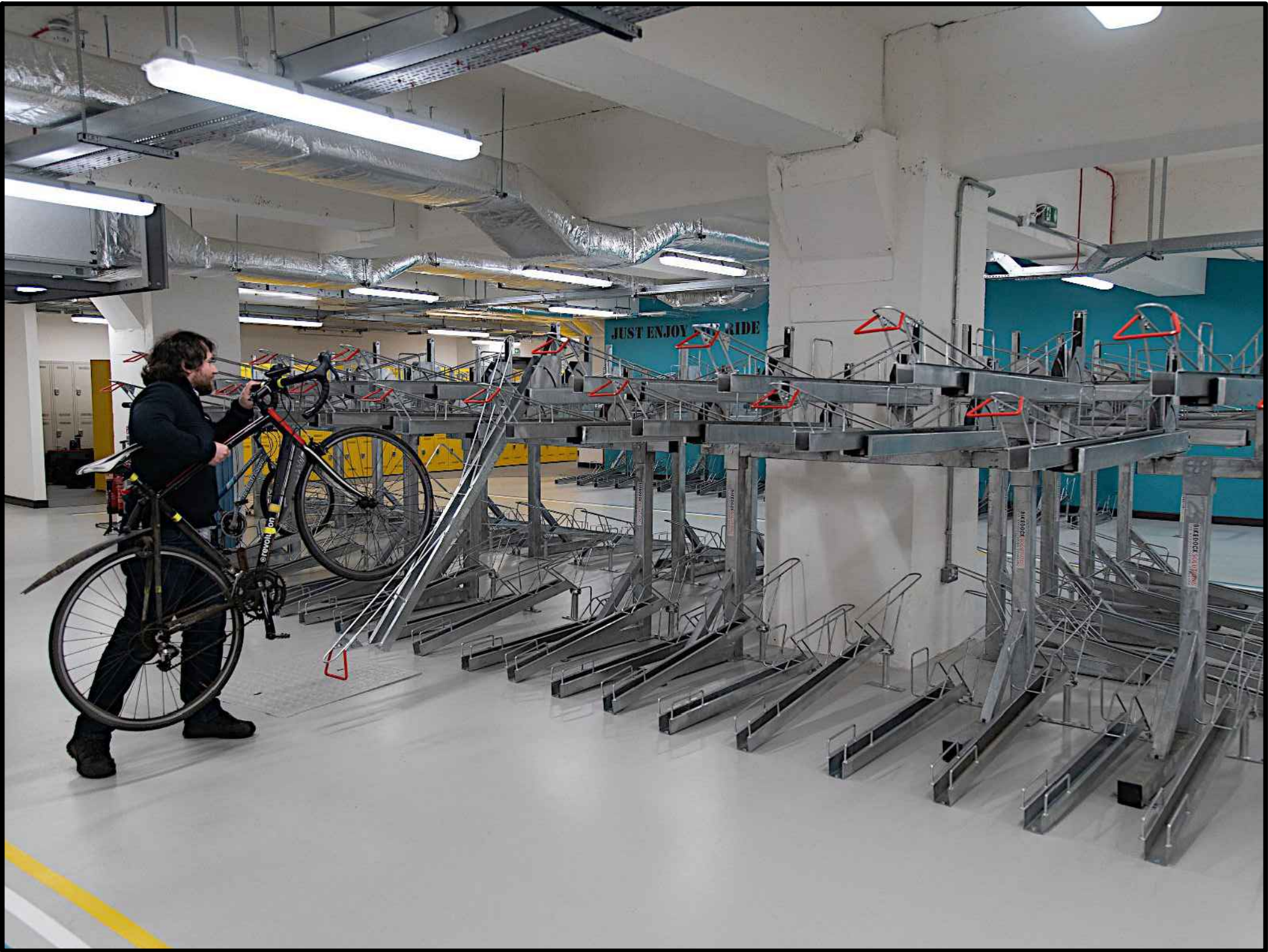
Bike Dock Solutions - Two Tier Bike Rack - Gas Assisted
