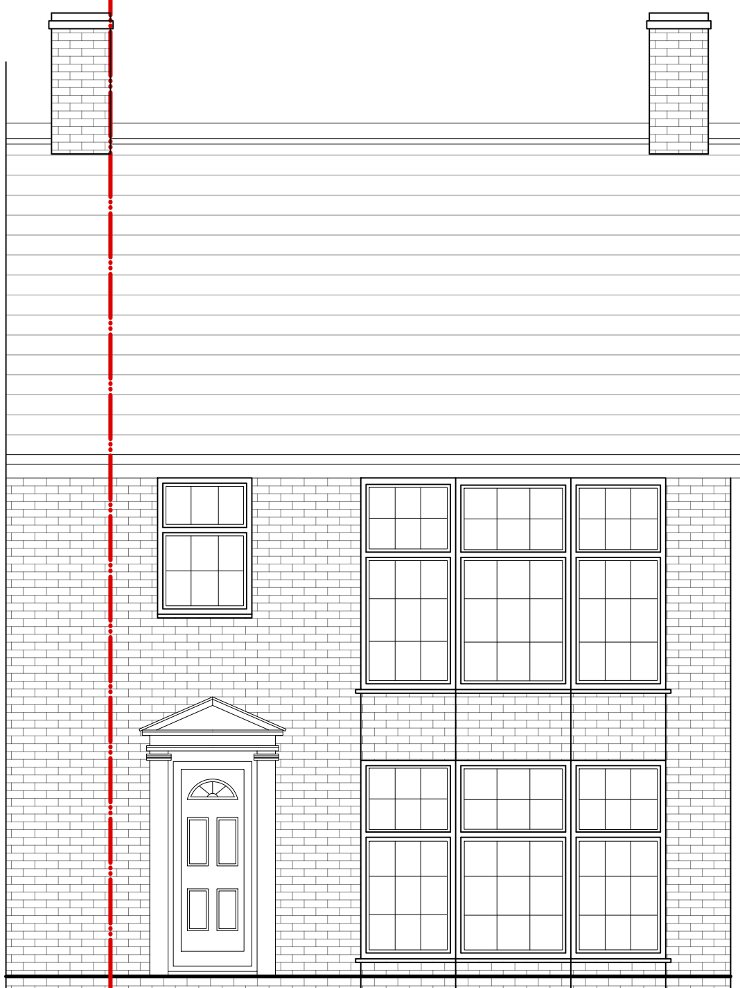
EXISTING SOUTH ELEVATION 1:50
