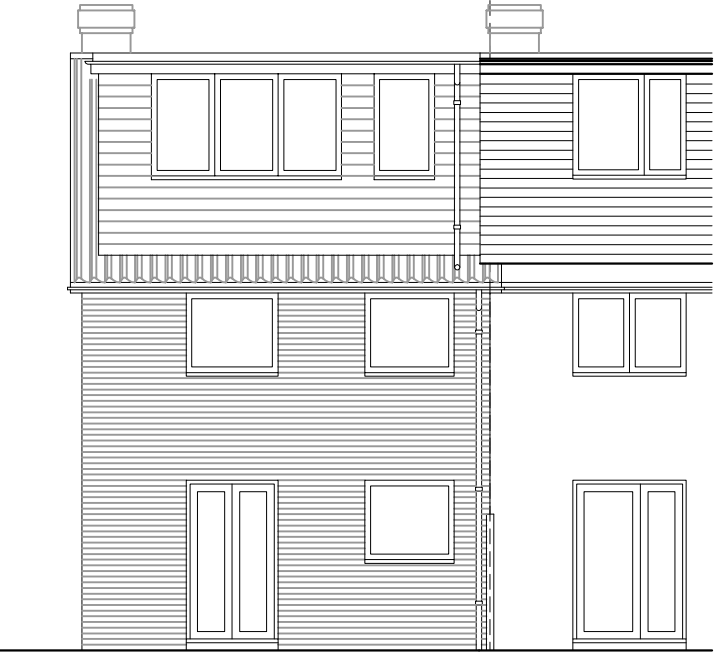
EXISTING NORTH-WEST FACING (REAR) ELEVATION 1:100
