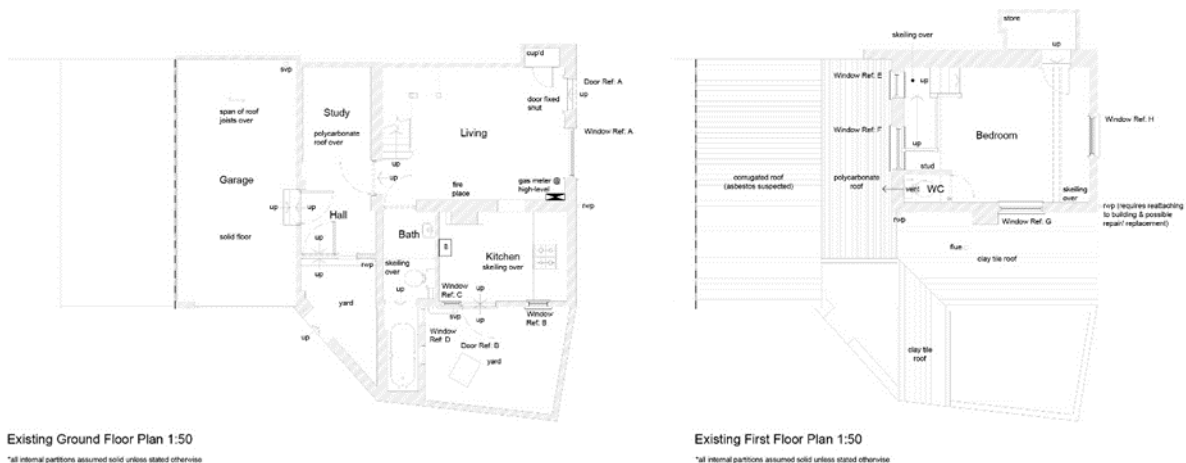
Image 05 – Existing Ground and First Floor Plans
