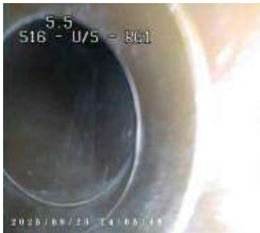
8c439efb-de48-4bea-a404-e04cdf25e8ec.png, 00:01:00, 5.50 m Line deviates up
