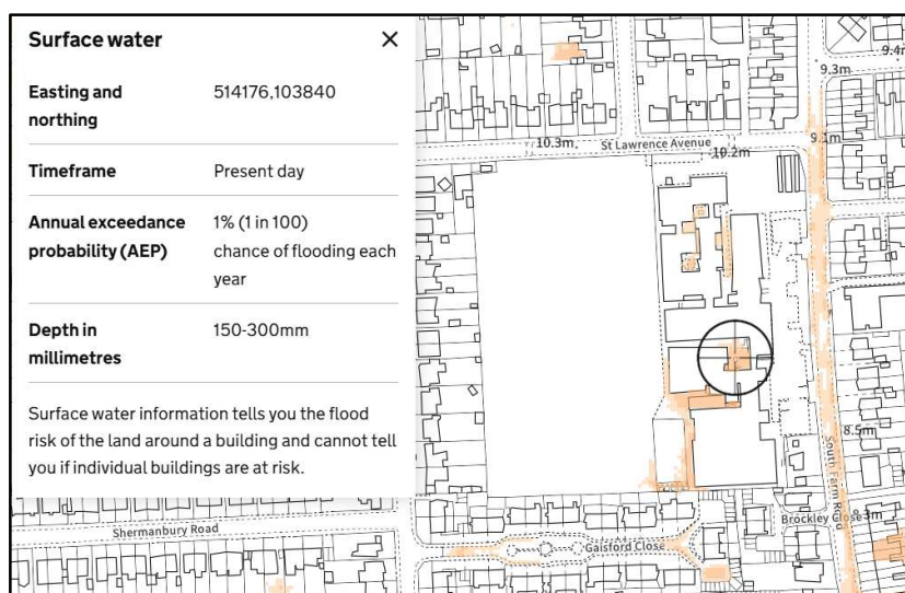
Figure 4 School Site showing risk of surface water flooding (at 1% chance) within existing buildings
