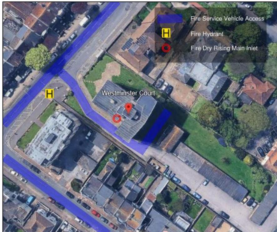
Figure 10 – Fire service access
