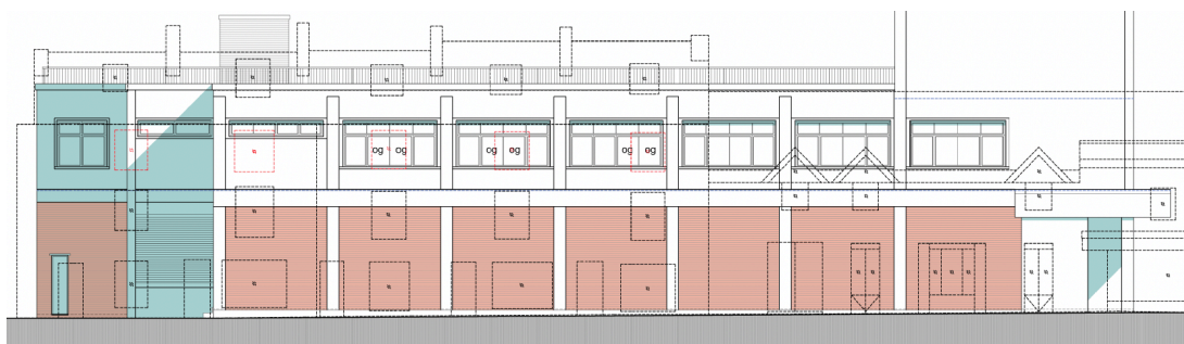
Figure 10 - Proposed east elevation with position of neighbouring windows shown dashed
