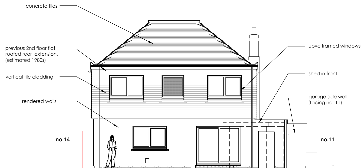
Existing North Facing Elevation (rear)
