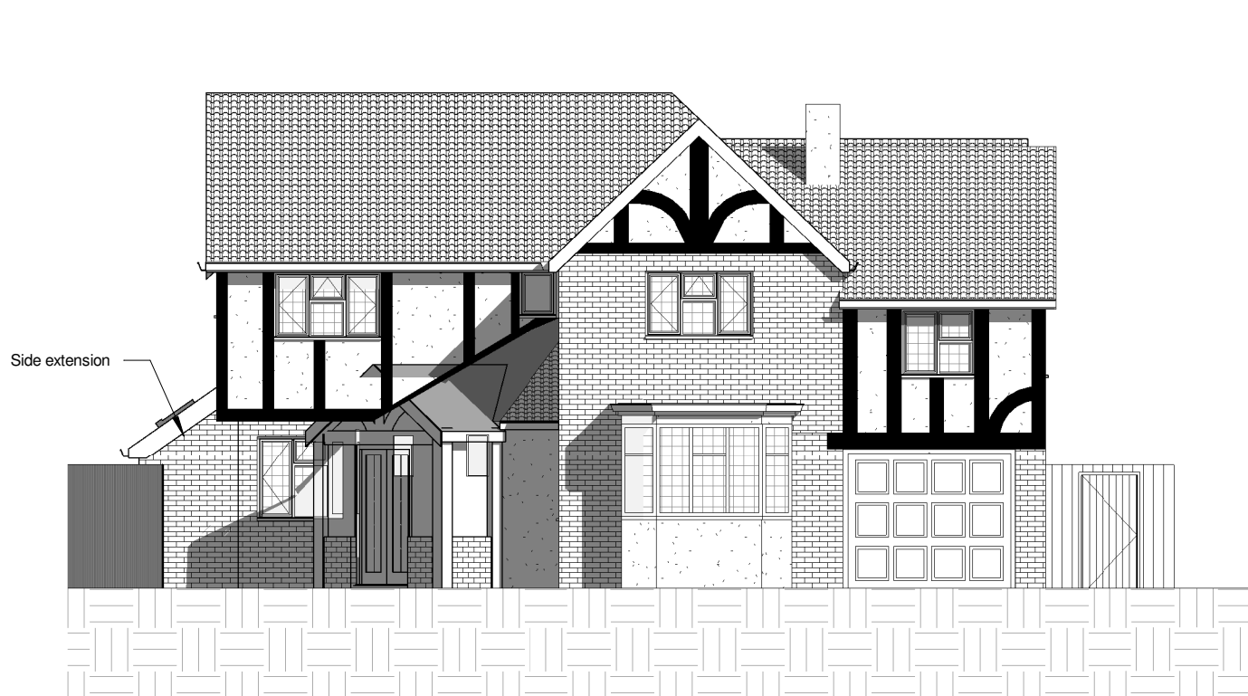
1 ELEVATION FACING EAST 1 : 100
