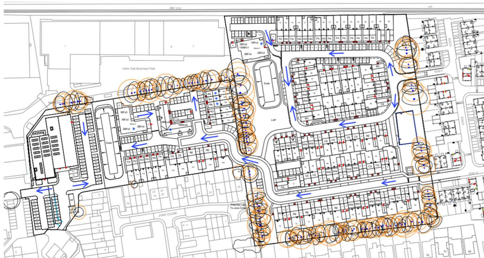
Figure 6-1 : Surface Water Flow Route Through the Development
