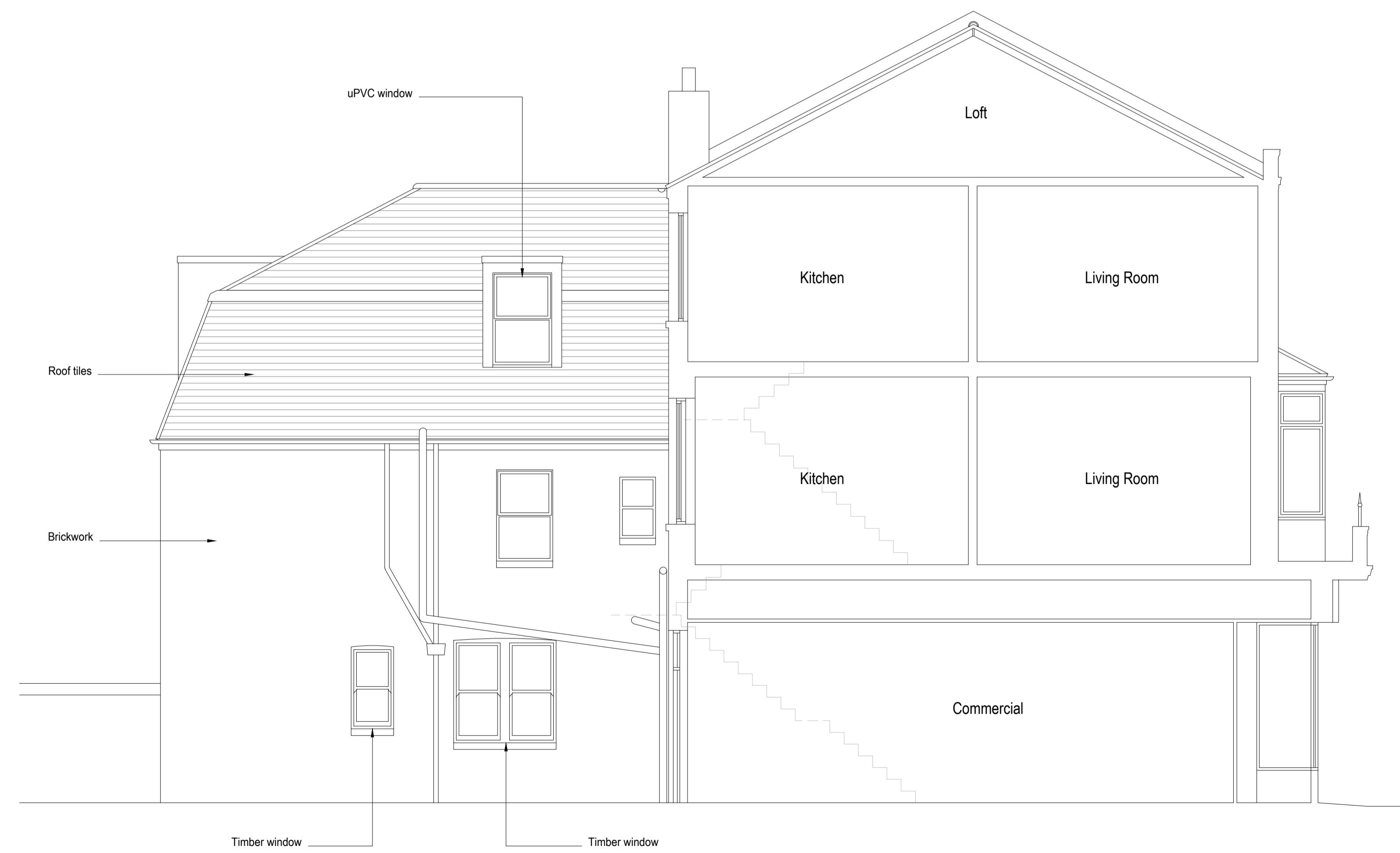
Existing Sectional Elevation A-A 1:50
