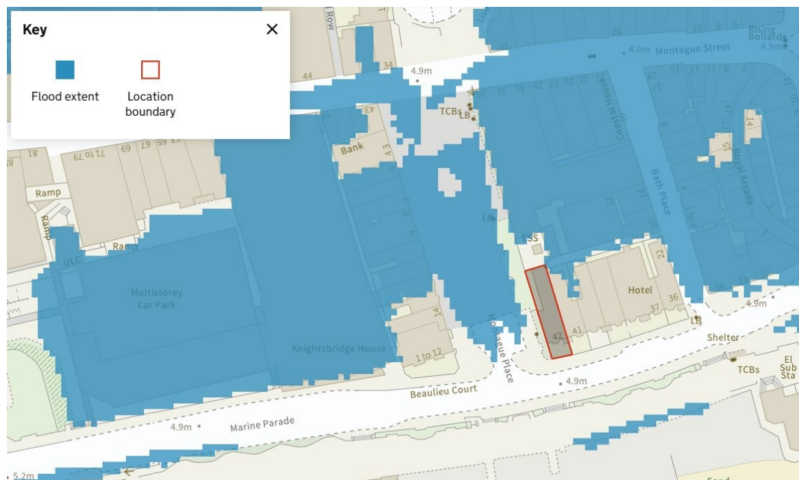
Figure 3: EA Risk of Flooding from Surface Water — 1 in 100 year (1% AEP) extent. The application site building footprint remains unaffected at this return period. Mapped extent widens along Montague Street and includes the open area between the building and the Bank to the north, with continued involvement of the Marine Parade carriageway and Multistorey Car Park. Source: gov.uk/check-long-term-flood-risk, extracted 5 May 2026.
