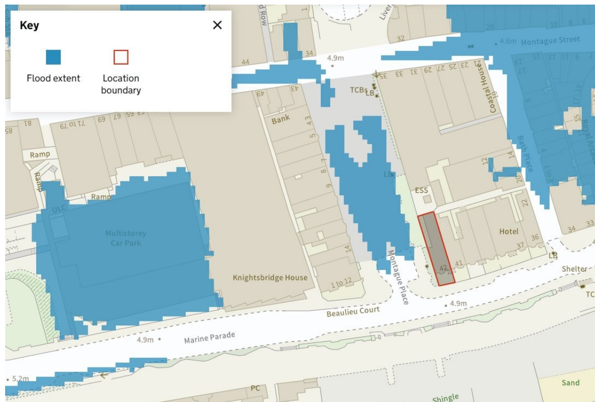
Figure 2: EA Risk of Flooding from Surface Water — 1 in 30 year (3.3% AEP) extent. The application site (red outline) is unaffected by mapped surface water at this return period. Flooding is confined to the Marine Parade carriageway corridor and the Multistorey Car Park area on the western side of Montague Place. Source: gov.uk/check-long-term-flood-risk, extracted 5 May 2026.
