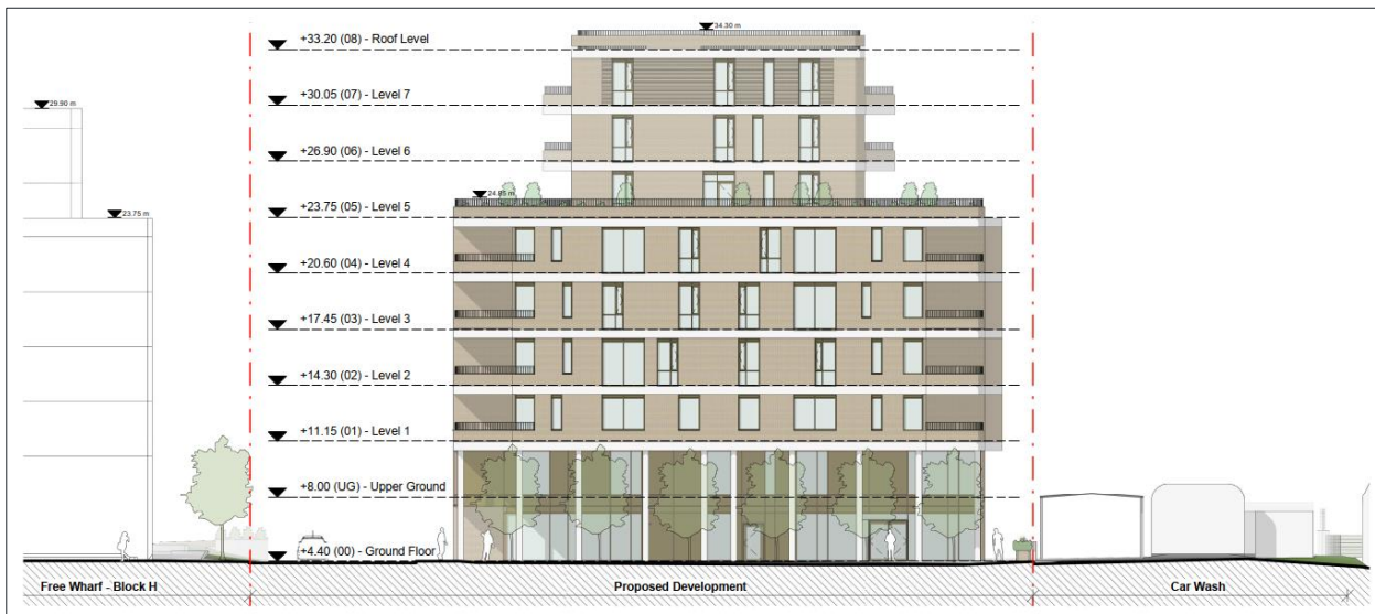
Figure 3 Floor levels and northern elevation
