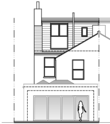
Proposed Rear Elevation (W) 1:100
