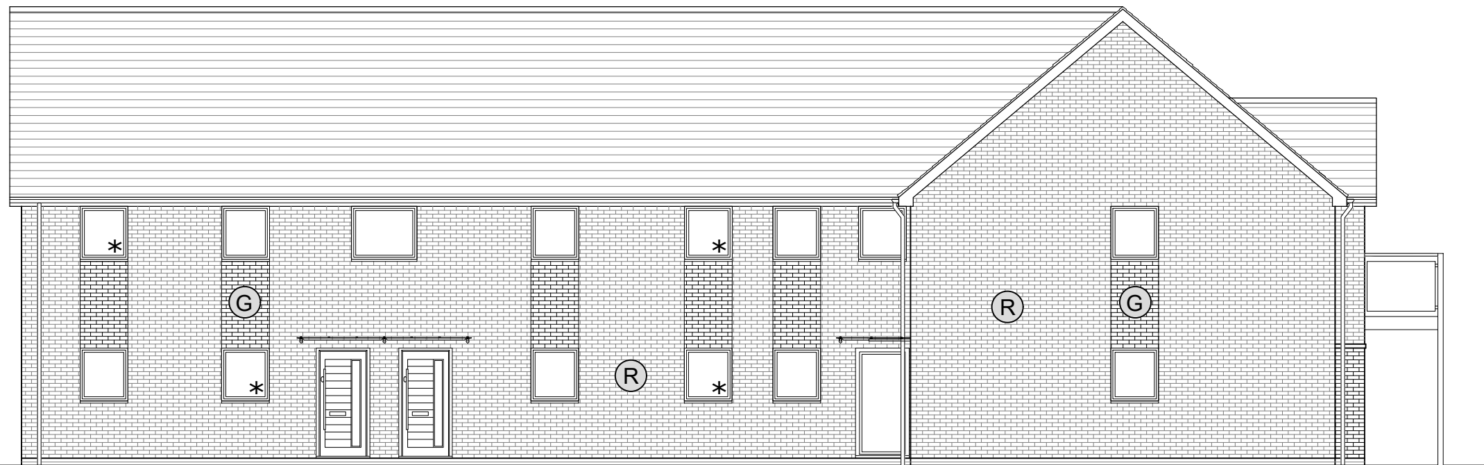
SIDE ELEVATION * Obscure Glazing
