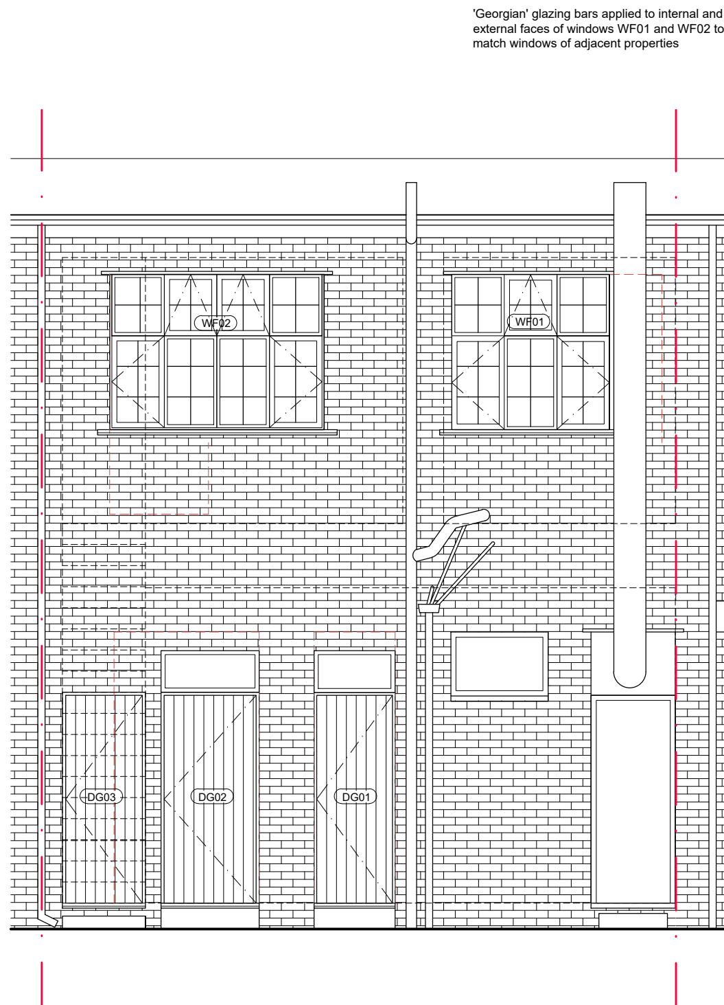
Rear Elevation - South-east facing (1:50)
